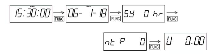
"The time elapsed from the previous correction" refers to the time elapsed after the last time correction was made by means of GNSS receiver (option), or external synchronization.
