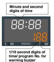
• Operation Procedure: Start of Timer (Ex.: Timer time: 10 minutes and 30 seconds, Program 1 for warning buzzer: 1 minute and 30 seconds, counting in 1/10 second increments)
